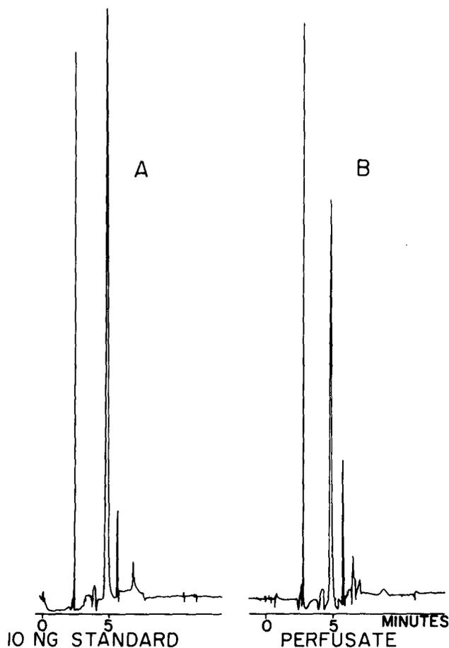
FIG. 1. Chromatograms of (A) 10 ng ascorbic acid standard and (B) perfusate. Retention time of ascorbic acid is 4.9 minutes. Conditions as described in text.
